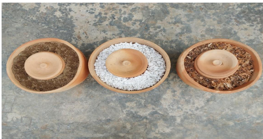
Fig. 3. Zeer pot refrigerators with different lining media
