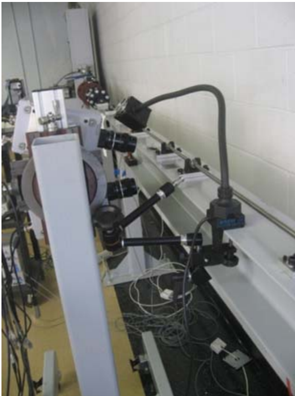
Figure 5. Digital image correlation set-up and lightning.
