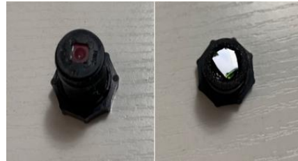
Fig. 3. Replacement of infrared filter bandpass filter instead
