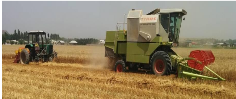
Fig. 2. A view of super straw management system attached behind the combine harvester and direct drilling of wheat seed by happy seeder [19]
