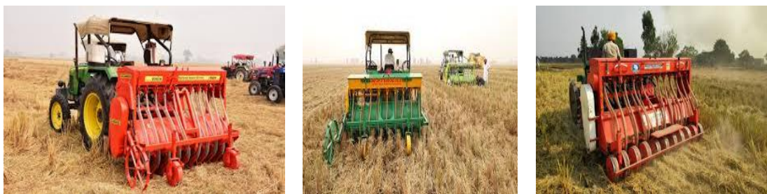
Fig. 4. A view of sowing of wheat seed by happy seeder in paddy residue retention
