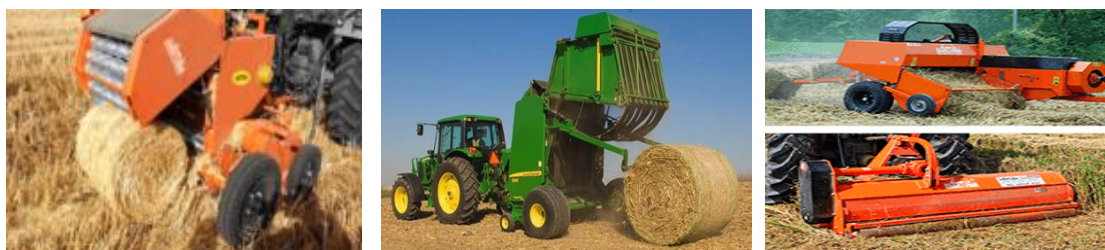
Fig. 5. A view of straw bailer for bailing of paddy / wheat straw in combine harvested field
