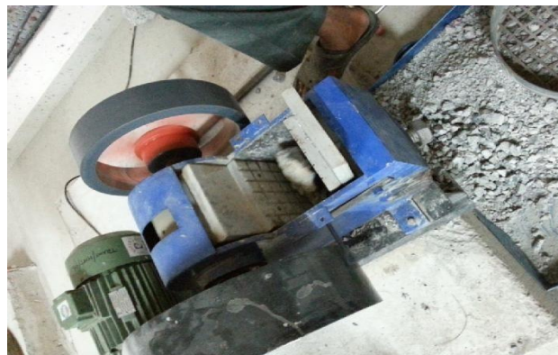
Fig. 7. The laboratory jaw crusher used for producing coarse recycled aggregate
