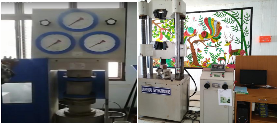
Fig. 10. Compressive test Machine and Universal test machine for finding
