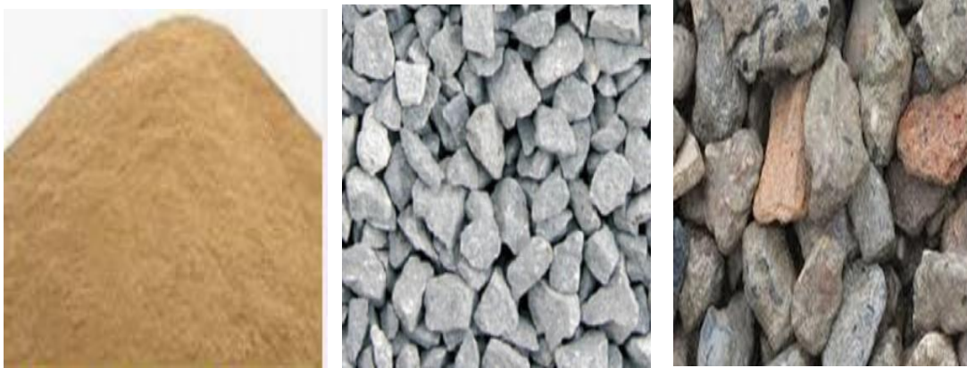
Fig. 8. Natural river sand; (b): machine crushed HG chips; (c): Recycled coarse aggt
