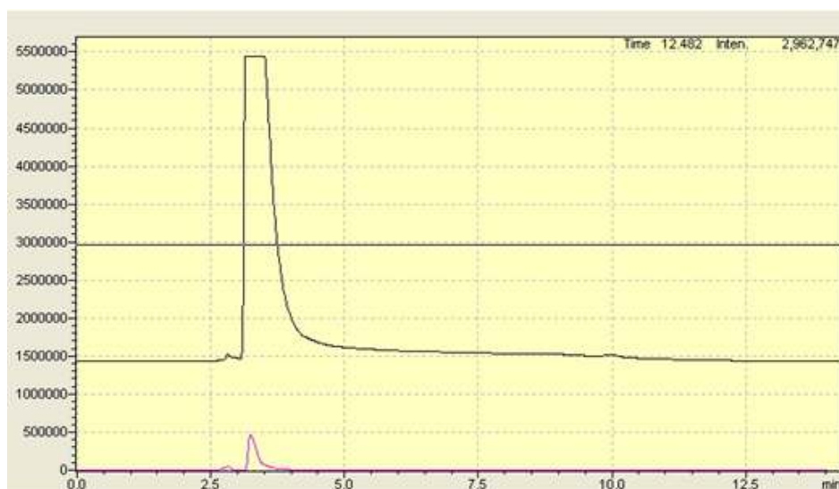
Fig. (1-b). Tracing the consumption of carbazole by HPLC in cell-free supernatant of bacterial culture
