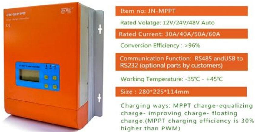
Fig. 6. Charger controller specification
