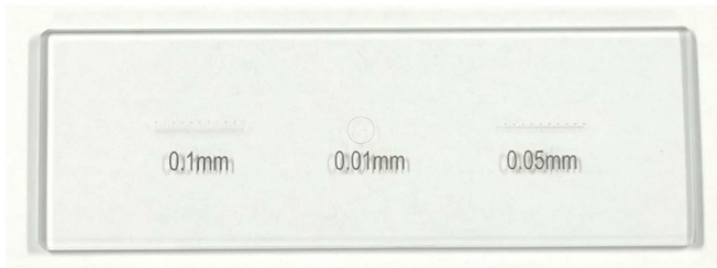
Figure 12. Physical map of the CW-DY objective micrometer. It has three standard scales: 10 mm subdivided into 100 cells, 1 mm subdivided into 100 cells and 10 mm subdivided into 200 cells.
