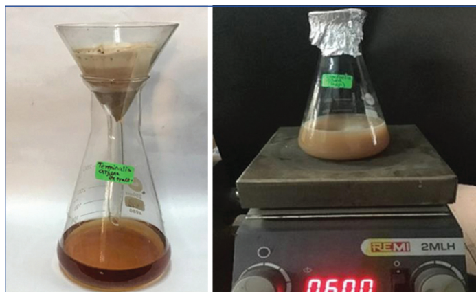
[Table/Fig-1]: Collection of purified plant extract post filtration using Whatman filter paper no.1.
