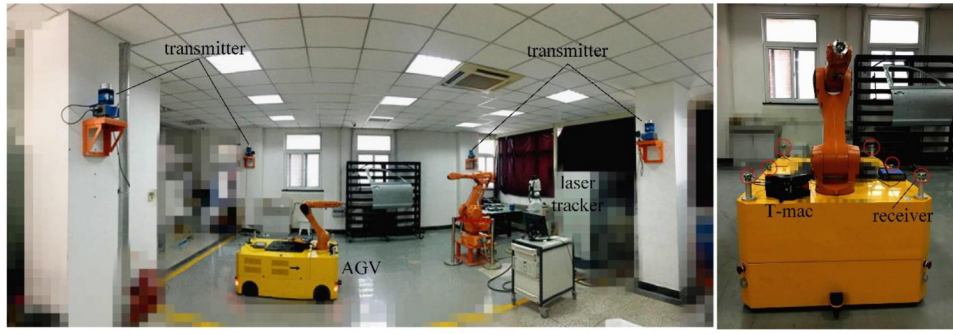
Figure 8. Experiment platform for dynamic 6-DOF measurement.
