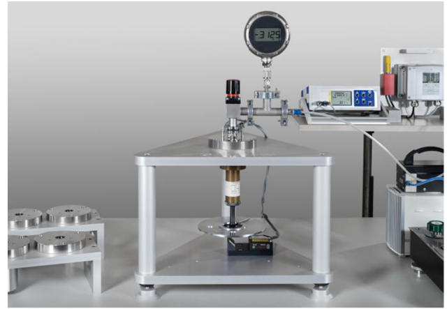
Figure 5. Set-up for operating piston-cylinder assemblies mounted upside-down.
