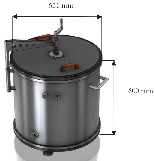
Figure 1. Hermetic chamber developed by CMI in which the standard instrument and device under test can be enclosed. A handle allows one to clamp the closing cover. Leaktight feedthroughs are used for pressure and electrical connections.
