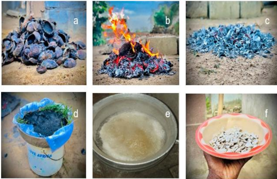
Fig. 8. Example of potash manufacturing technology based on cocoa pods a – Collection of the co-products; b – Incineration of the co-products; c - collection of ashes; d - the wetting of the ash with water and the dripping of wet ashes; e- The preparation of the supernatant; f - collection of potash after solidification
