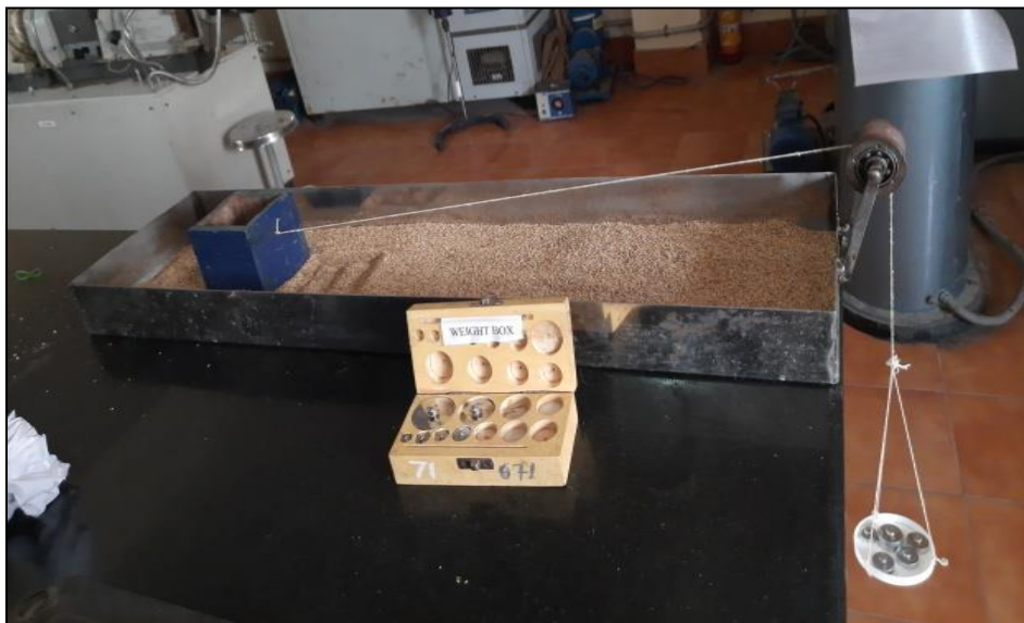
Fig. 2. Measurement of frictional properties of foxtail millet seeds
