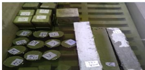
Fig. 4. Compressive, splitting and flexural concrete samples during curing
