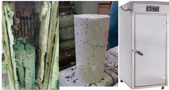
Fig. 9. Specimens exposed to temperature in electric oven drier
