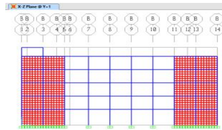
Fig. 17. Modelling of shear wall in direction XZ
