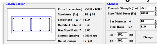
Fig. 26. Design of Selected Column Due to gravity loads & seismic loads after strengthening adding RC shear walls
